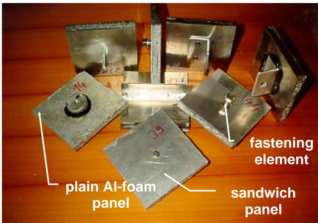
**Figure 5: Aluminium foam samples with various fastening elements**
