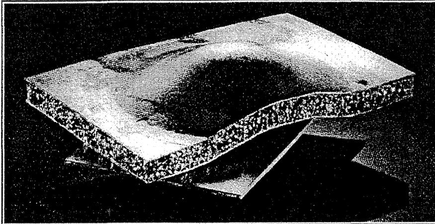
Figure 4: Metal foam sandwich before and after foaming
