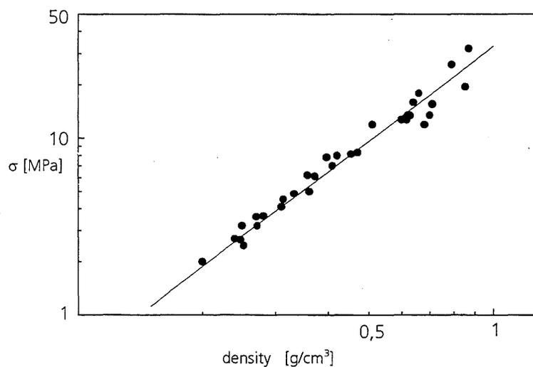
Figure 6: Compression strength of a series of AlSi12 foams.
