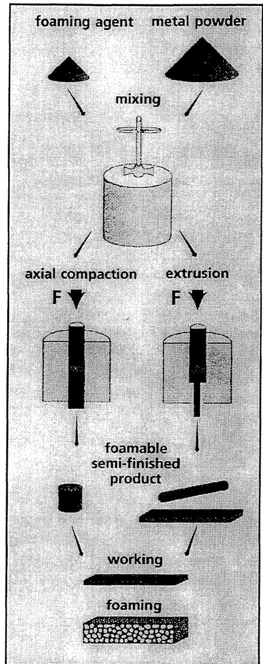
Figure 1: Powder metallurgical production method of metal foams
