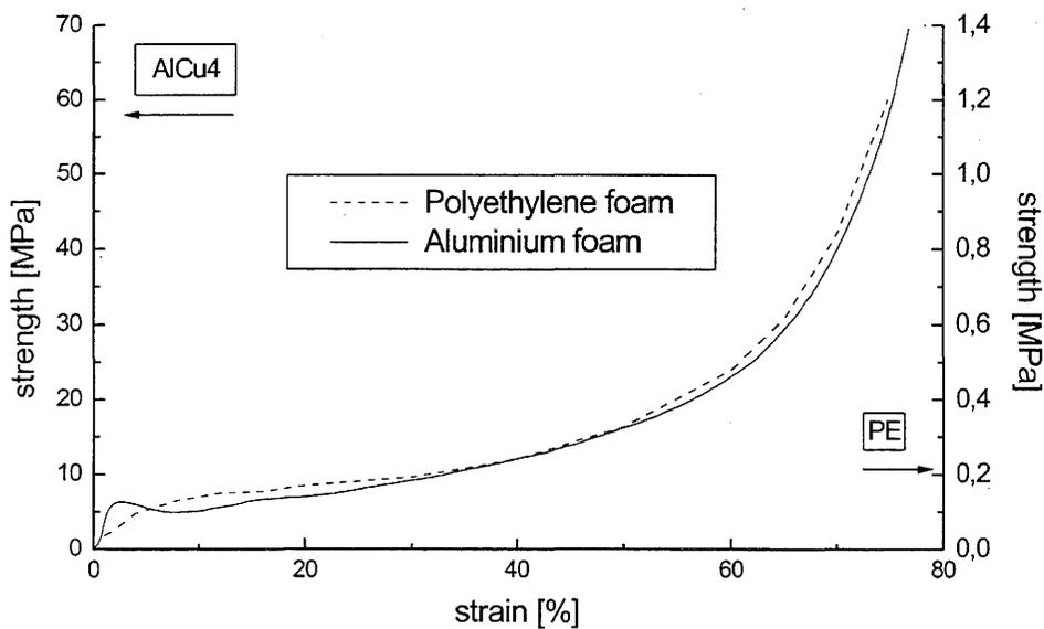
Figure 5: Loading curves of aluminum and polyethylene foams.
