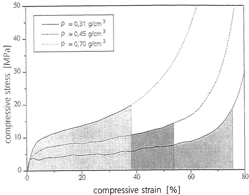
Fig. 7: Loading curves of three Al foams
