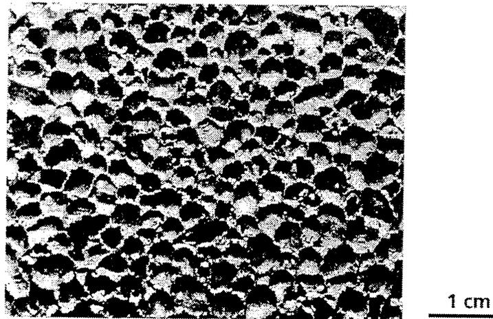
Figure 2: Typical aluminum foam microstructure.
