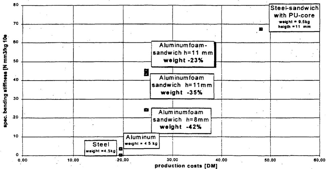
Figure 8: Potential for weight reduction and production costs in automotive applications
