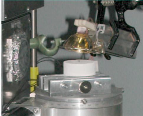
Figure 12: Heating set up for tomography on liquid foams, consisting of a heating lamp and a sample holder made of refractory clay. A thermocouple is located directly beneath the sample.
