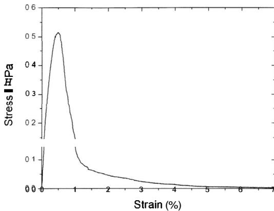
Fig. 3: Tensile stress-strain curve of the large foam sample (50x50x50 mm) with 4.0% relative density.
