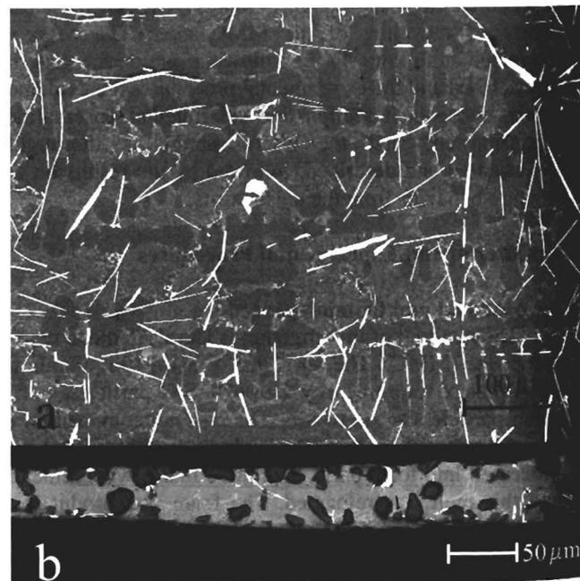
**Fig. 2: (a) BSE image of an embedded and polished cross-section of a strut showing the microstructure. Dendrites of a-Al and eutectic structure of Al-Si with needles of  $\beta$ -AlFeSi (white) (b) Embedded and polished cross-section of a cell wall. The dark inclusions are the SiC particles.**
