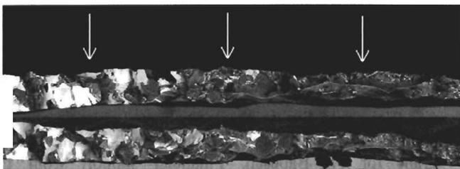
Fig. 4: Fracture surfaces of a cell wall width. Left arrow indicates cleavage of a  $\beta$ -AlFeSi plate. Middle arrow indicates fractured SiC particles and dimples with Si and the right arrow indicates ductile Al fracture. Upper fracture surface is mirrored for convenience.
