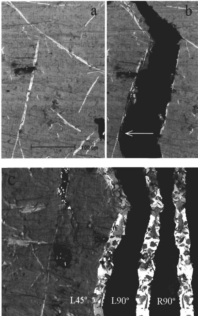
Fig. 6 (a) BSE image of the area marked by the black square in fig. 5a, prior to deformation. (b) After deformation, white arrow indicates the point of initiation. (c) Left fracture surface at 45° and 90° and the right fracture surface at 90°
