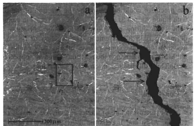
Fig. 5: (a) BSE image of the cell wall used in the in-situ tensile test prior to deformation. Black square indicates the area of figure 6. (b) Cell wall after deformation. Black arrows indicate initiation points.
