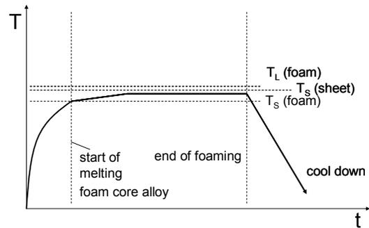
Figure 4. AFS foaming in a regulated furnace.
