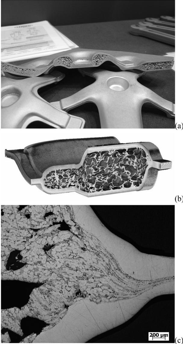
Figure 5. Forged AFS, (a) part and section, (b) tomogram of interior (courtesy F. Garcia-Moreno), (c) microstructure of densified rim.
