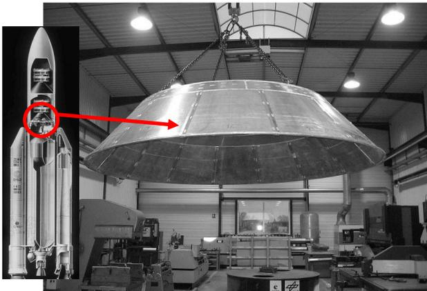
Figure 7. Ariane 5 rocket cone prototype made of AFS.
