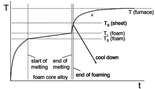
Figure 3. Temperature course of AFS foaming in an unregulated furnace.
