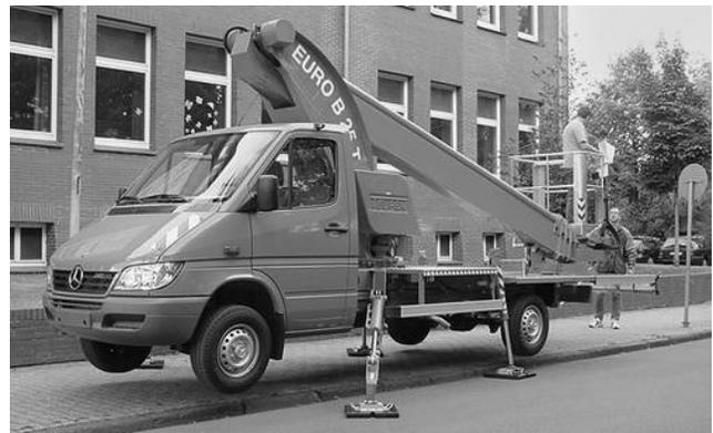
Figure 6. Vehicle with ‘EURO B25T’ lifting arm support.
