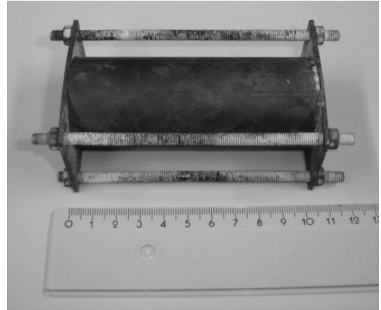
FIGURE 1: Cylindrical mould used for different foaming configurations.
